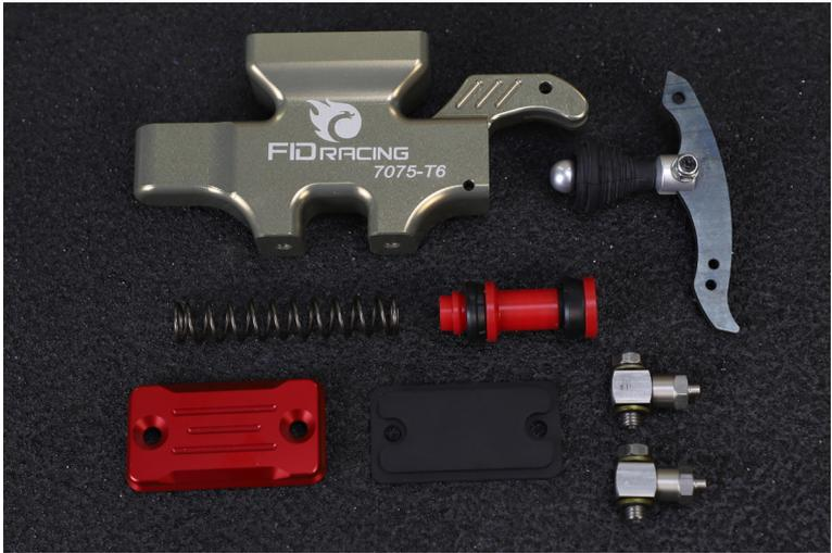
Master pump is made of high strength alloy 7075-T6, CNC machined in high precision and hard-anodized. It is dual Y-ring piston design. Piston shaft is red POM material, with excellent strength and anti-friction property. Others include stainless steel tube connectors, HRC60° 65Mn spring brake pedal, piano-wire return spring.
