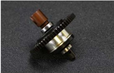
**Central Differential:** Small crown gears is made in powder metallurgy method. Spur gear is made of 20CrMnTi gearing steel via CNC. Diff housing is made of aluminum alloy 6061-T6. 60T big gear and 2 × covers are made of 45#steel (equivalent to US 1045 steel and Europe C45 steel) via CNC, surface black-oxided. Drive cup in 65Mn spring steel. Differential Lubricant in 50000cSt.
