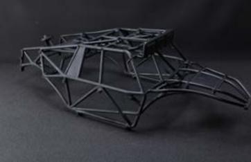
**Body Shell & Roll Cage:** Body shell is made of 1.5mm thick PC material. Roll cage is made of 10mm diameter rod in high-strength nylon PA6 material.
