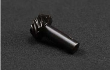
**Front Gearbox:** Gearbox housing is made of aluminum alloy ADC12 in die casting method. Small helical crown gear is made of 20CrMnTi gearing steel via CNC, and surface black-oxided. Gear ratio in 13T: 43T, and gear module in 1.5M.
