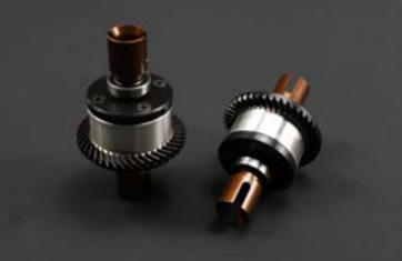
**Front & Rear Differential:** Small crown gears is made in powder metallurgy method. Big helical crown gears is made of 20CrMnTi gearing steel via CNC. Drive cup is made of 65Mn spring steel, PIN in 5mm diameter, housing in aluminum alloy 6061-T6, differential lubricant in 50000cSt.
