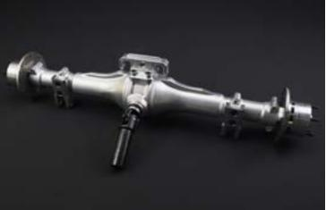
**Solid Rear Axle:** Rear axle housings are made of one-piece aluminum alloy 6061-T6 via CNC, and decorated with beautiful line pattern. Wheel comes with 4mm thick brake disc compatible with FID Racing hydraulic braking system. Inside the axle is a metallic differential as introduced above. Wheel hub comes with 5 × lugs adapter, stable and real-life.
