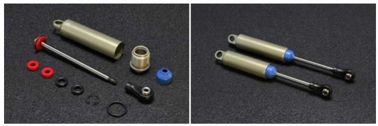
Front & Rear Hydraulic Dampers: Damper bodies are made of aluminum alloy 7075-T6, with better abrasion resistance. Inner plugs are made of best Polyoxymethylene (POM) material, with good abrasive resistance and strength. Dual seal ring design, 7mm dia. damper shaft. Working with shock to provide best shock absorbing effect.
