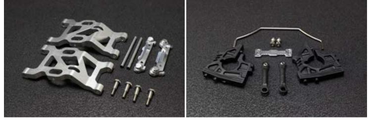
**Front Arm:** Arm and arm braces are made of aluminum alloy 6061-T6. Arm PIN upgrades to 7mm diameter and is made of hard chrome steel GCr15. Nylon gearbox braces (optional metallic braces) and 4mm diameter swaybar.
