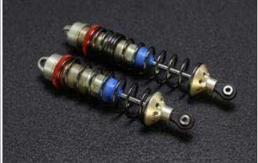
Front & Rear Hydraulic Shocks: Shock bodies are made of aluminum alloy 7075-T6 with better abrasion resistance. Inner plugs are made of best Polyoxymethylene (POM) material, as well with good abrasive resistance and strength. Dual seal ring design, 7mm dia. shock shaft, springs made of 3mm diameter music wire, treated with hardening process and black-oxidation. Rear shock consists of two springs.
