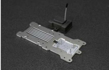
**Steering & ESC Mount:** Ackermann steering system design, automatic return-to-center, servo protection mechanism against big impact or too much turning force. ESC mount is made of aluminum alloy 6061-T6.
