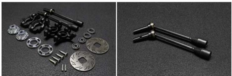
**Front Wheel System:** Spindle carrier is made of nylon PA6. 4mm thick brake disc comes in standard configuration and is compatible with FID Racing hydraulic braking system. Front wheel drive shaft is made of 45# steel (equivalent to US 1045 steel and Europe C45 steel), heat treated and black-oxided. 5mm PIN for drive axle cup. 5 × lugs wheel adapter in aluminum alloy 6061-T6.
