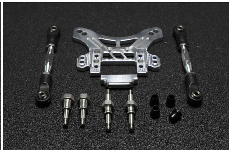
Front & Rear Shock Towers: Shock towers are made of aluminum alloy 6061-T6 via CNC. Rear swaybar is redesigned and upgrades to 4.5mm diameter. Shock and damper mount in stainless steel.
